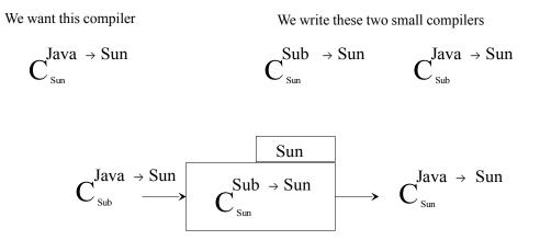
Figure 1.7 Bootstrapping Java onto a Sun Computer
