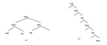
**Figure 2.8** (a) A Balanced Binary Search Tree (b) A Binary Search Tree Which is Not Balanced
