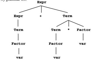
Figure 3.9 A Derivation Tree for var + var \* var Using Grammar G5
