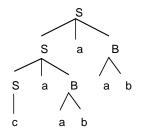
Figure 5.1 A Derivation Tree for the String caabaab, Using Grammar G19
