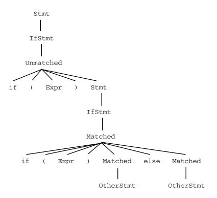
Figure 3.11 A Derivation Tree for if (  ${\tt Expr}$  ) if (  ${\tt Expr}$  ) OtherStmt else OtherStmt using Grammar G7
