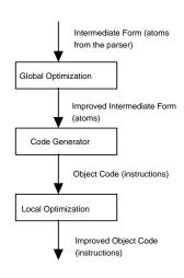
**Figure 7.1** Sequence of Optimization Phases in a Compiler
