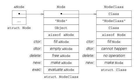
Here is a picture describing the linkage of exec() and new():
