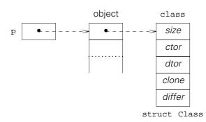
The type description **class** at the right is initialized at compile time. The object is created at run time and the dashed pointers are then inserted. In the assignment
