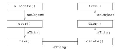
There is a balance: **allocate()** and **free()** deal with the same region of memory; by default, **new()** gives it to its constructor, **delete()** to its destructor; and the constructor and destructor only deal with resources represented inside the object. **new()** and **delete()** should only be overwritten to interfere with the flow of memory from **allocate()** to **free()**.
