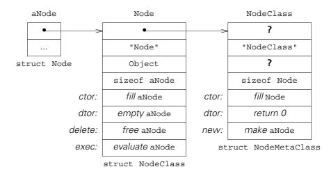
With this arrangement we can give **new()** dynamic linkage for the call
