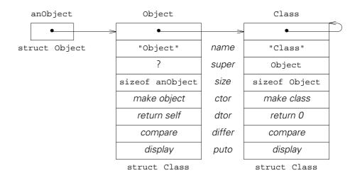
The question mark indicates one rather arbitrary decision: does **Object** have a superclass or not? It makes no real difference, but for the sake of uniformity we define **Object** to be its own superclass, i.e., the question mark in the picture is replaced by a pointer to **Object** itself.
