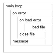
In this case we need two **longjmp()** targets for recovery: **onError** returns to the main loop and **onLoadError** is used to clean up after a bad loading operation:
