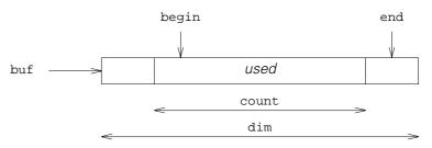
**begin** and **end** limit the used part of the list, **dim** is the maximal buffer size, and **count** is the number of elements currently stored in the buffer. **count** makes it easy to distinguish between a full and an empty buffer. Here is the class description *List.d*:
