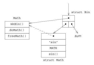
We let the left side of a binary node point to the symbol table element for the function and we attach the argument tree at the right. The binary node has **Math** as a type description, i.e., the methods **doMath()** and **freeMath()** will be called to execute and delete the node, respectively.
